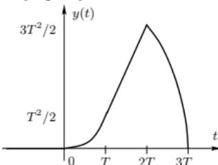
$$y(t) = \frac{t^2}{2}u(t) - \frac{1}{2}(t-T)^2u(t-T) + (2T^2 - \frac{1}{2}t^2)u(t-2T) + (\frac{1}{2}t^2 - tT - \frac{3}{2}T^2)u(t-3T)$$
