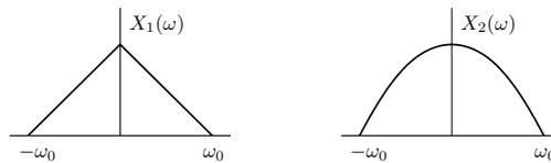
$$X_1(\omega) = X_2(\omega) = 0 \quad |\omega| > \omega_0$$
